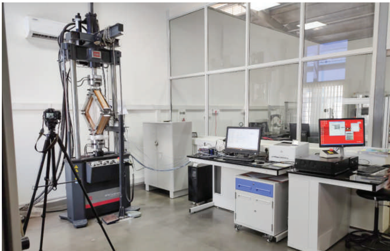
▀ A view of Structural Engineering laboratory with 100kN UTM and DAQ system
