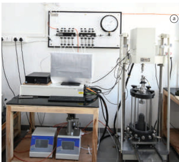
a. Automated electro-mechanical 20 kN actuator cyclic triaxial apparatus
