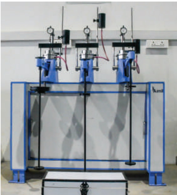
3-gang Oedometer setup
